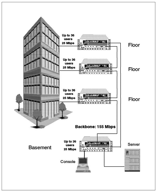
Figure 13. 8285 Low-Cost Configuration Implementation
